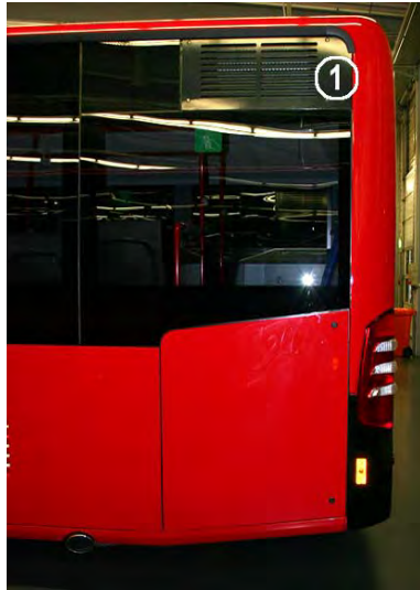
Air intake, upper
