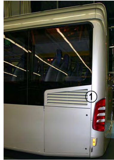
Air intake, centre
