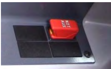
Pull up the flap, pull up the yellow switch
