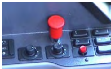
Unlock the red switch by turning it anti-clockwise
